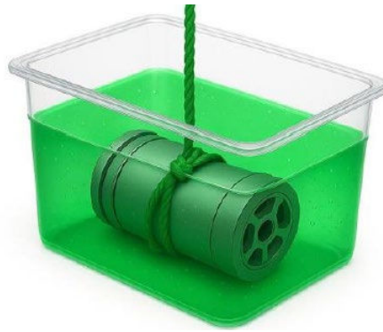
Fig. 7— Image representing an AVLST valve immersed in a 31% HCL acid bath for 2 hours
