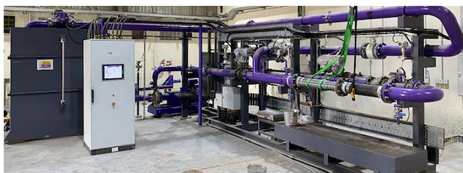
Fig. 6— API 10F flow loop used for the flow durability test
